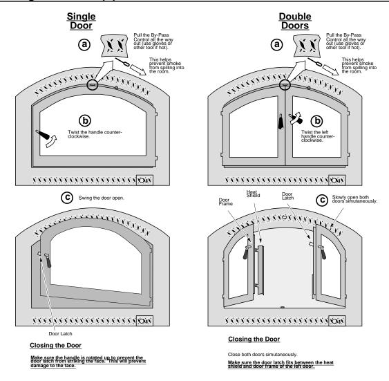
**Warning**: When closing the doors, make sure the door latch does not strike the front of the left side door. This will damage the finish on the doors.
